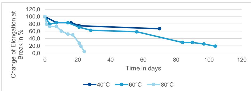
Change of elongation of break of Ultrasint® TPU 88A over time of water exposure
