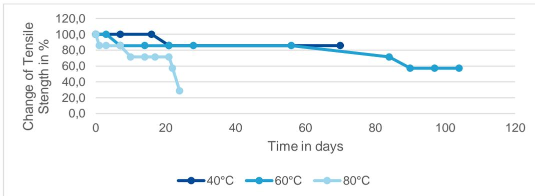
Change of tensile strength of Ultrasint® TPU 88A over time of water exposure
