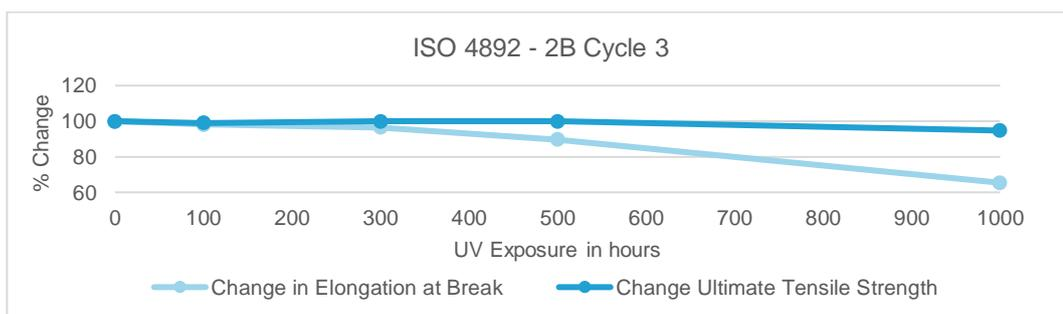
ISO 4892 – 2B Cycle 3 Change of mechanical properties over of 1000 hours of UV exposure
