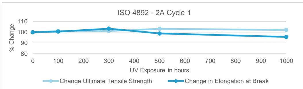
ISO 4892 – 2A Cycle 1 Change of mechanical properties over of 1000 hours of UV exposure
