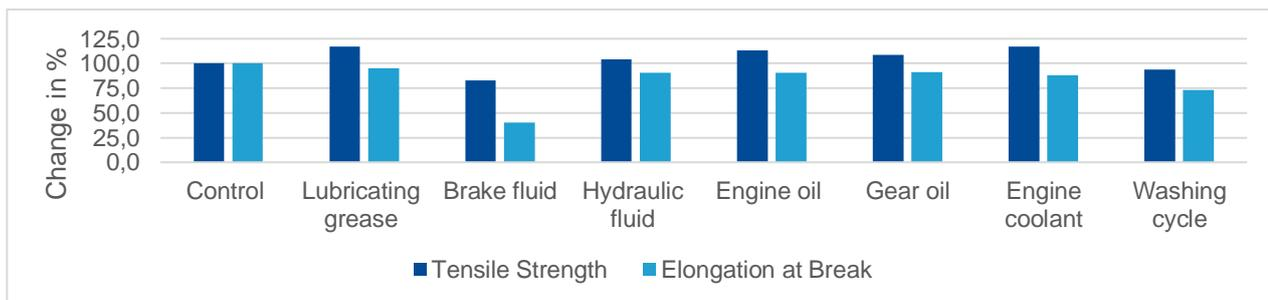
Change of mechanical performance of Ultrasint® TPU 88A due to exposure of chemicals
