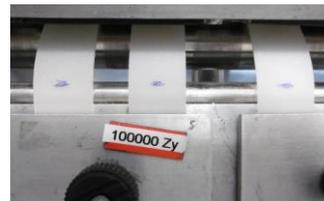
*Test set-up of Ross flex measurement of Ultrasint® TPU 88A*
