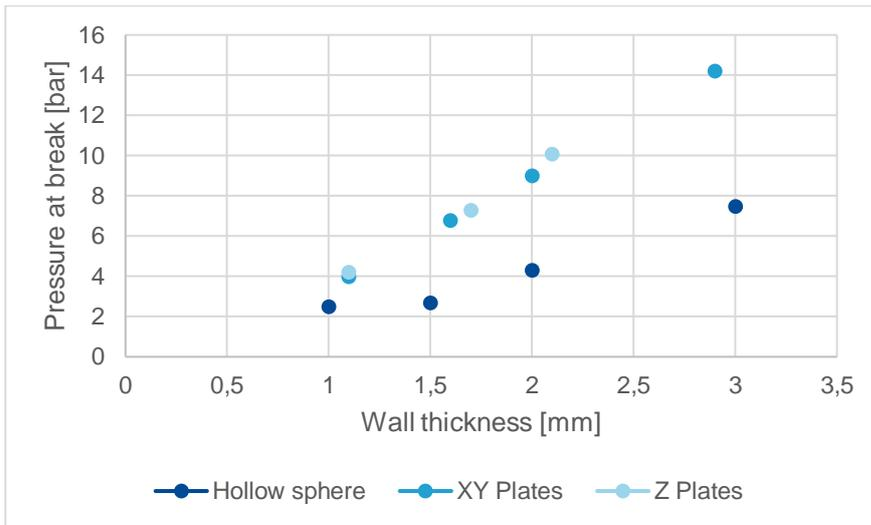
*Burst pressure of various geometries in Ultrasint® TPU 88A*
