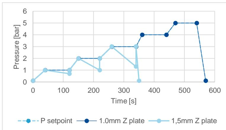
*Air tightness of various geometries in Ultrasint® TPU 88A*
